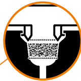
Filling Chamber properly filled
