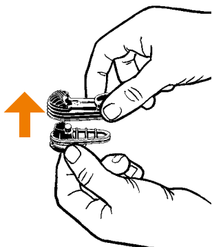
Pull the Cooling Unit Cap from the Cooling Unit Base
